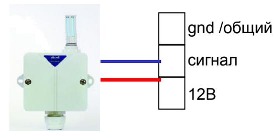
**Two wires connection, power supply+signal 4...20mA.**
