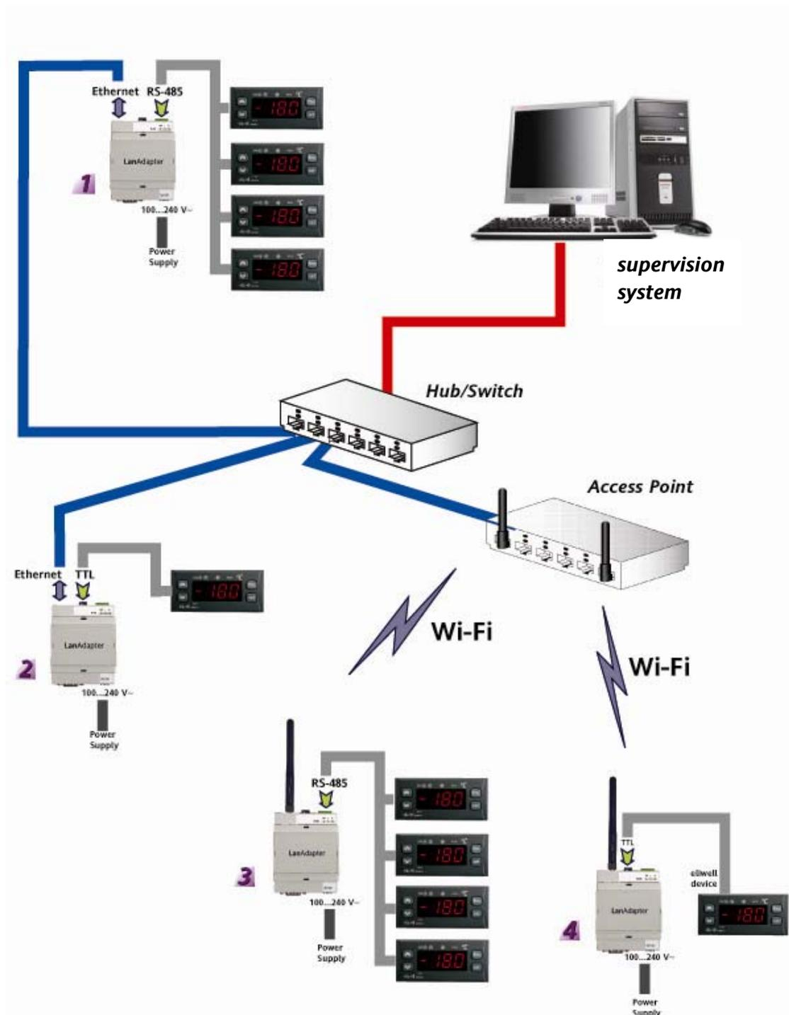
The network comprises a supervision system installed on a PC located within a LAN network. The following is a description of the 4 different installation methods used in the example network.
