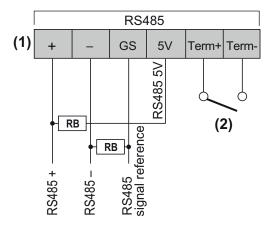
(1) (CN1) 5 V power supply for any external polarizing resistors (RB). Maximum current: 10 mA.
