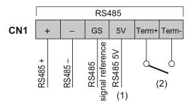
NOTE: the GS pin is not directly connected to the DC power supply connection of the "-" pin for the power supply unit.
