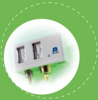
T.Ü.V. bellows are available on certain high pressure models. In this configuration the models incorporate a "bellows within a bellows", designed so that if the operating bellows develops a leak, the second bellows contains the refrigerant and shuts off the system. Braze connection versions are available with or without capillary.
