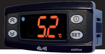
User terminal for full display and programming of controllers for ducted and plug-in refrigerated cabinets. Each power board can be connected to a single KDEPlus keypad and if required to an ECHO module for remote display by means of the connector located on the keypad. The keypad is not compatible with IWP series instruments.
