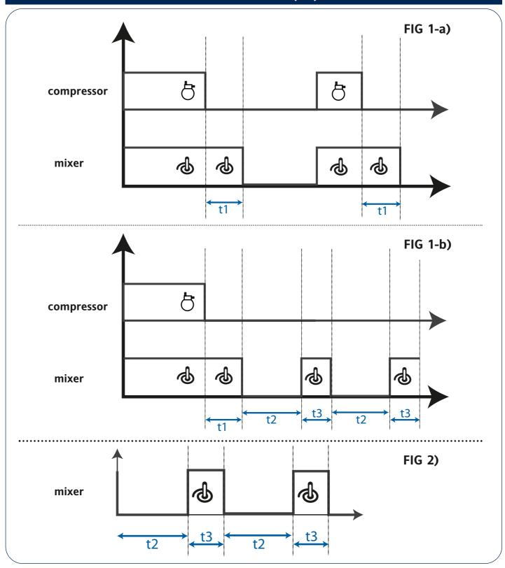
The Milk Controller **(MC)** function to run a milk mixer is managed by parameters in MC folder. There are 2 operating modes (determined by parameter **AtP**):
