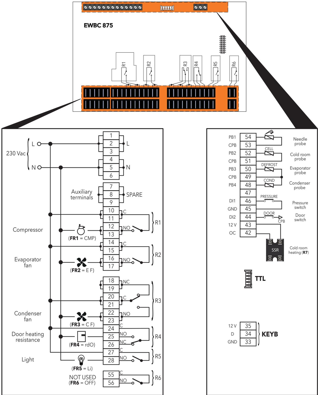
Fig. 11. EWBC 875 connection diagram example
