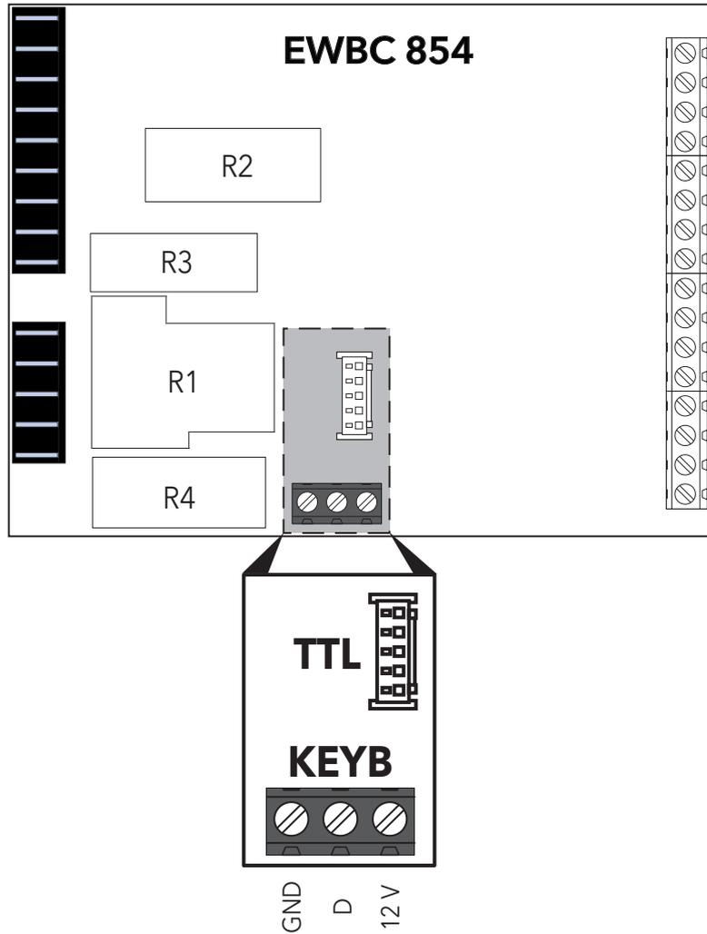
**Fig. 3.** Serial ports: TTL and KEYB
