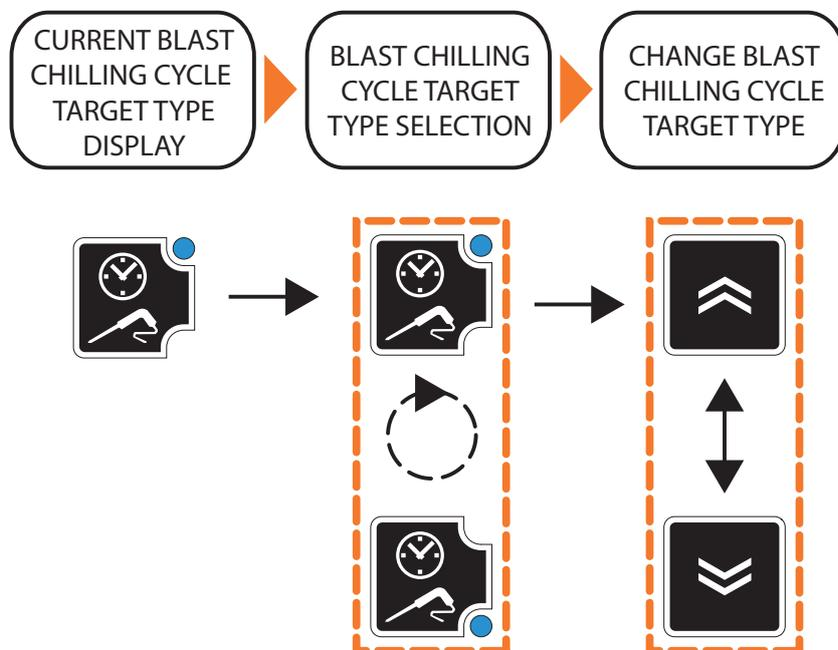
**Fig. 18.** Selecting a blast chilling cycle target type
