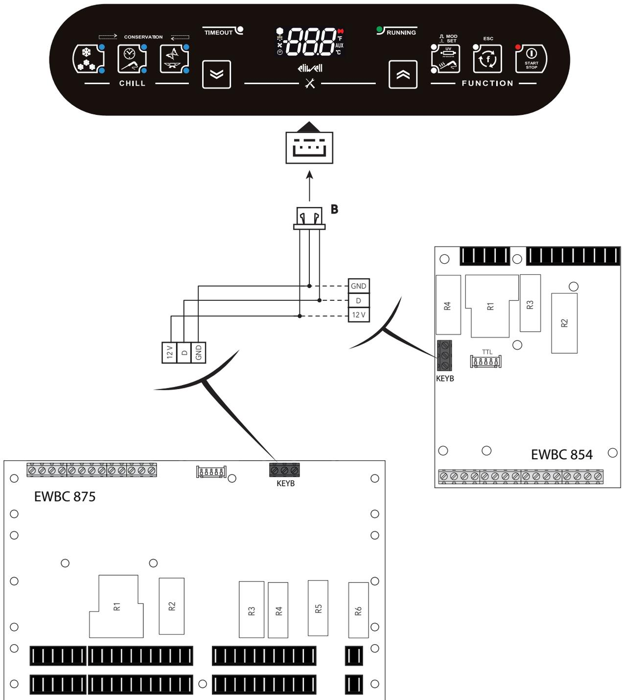
Fig. 9. Base boards and user interface connection diagram
