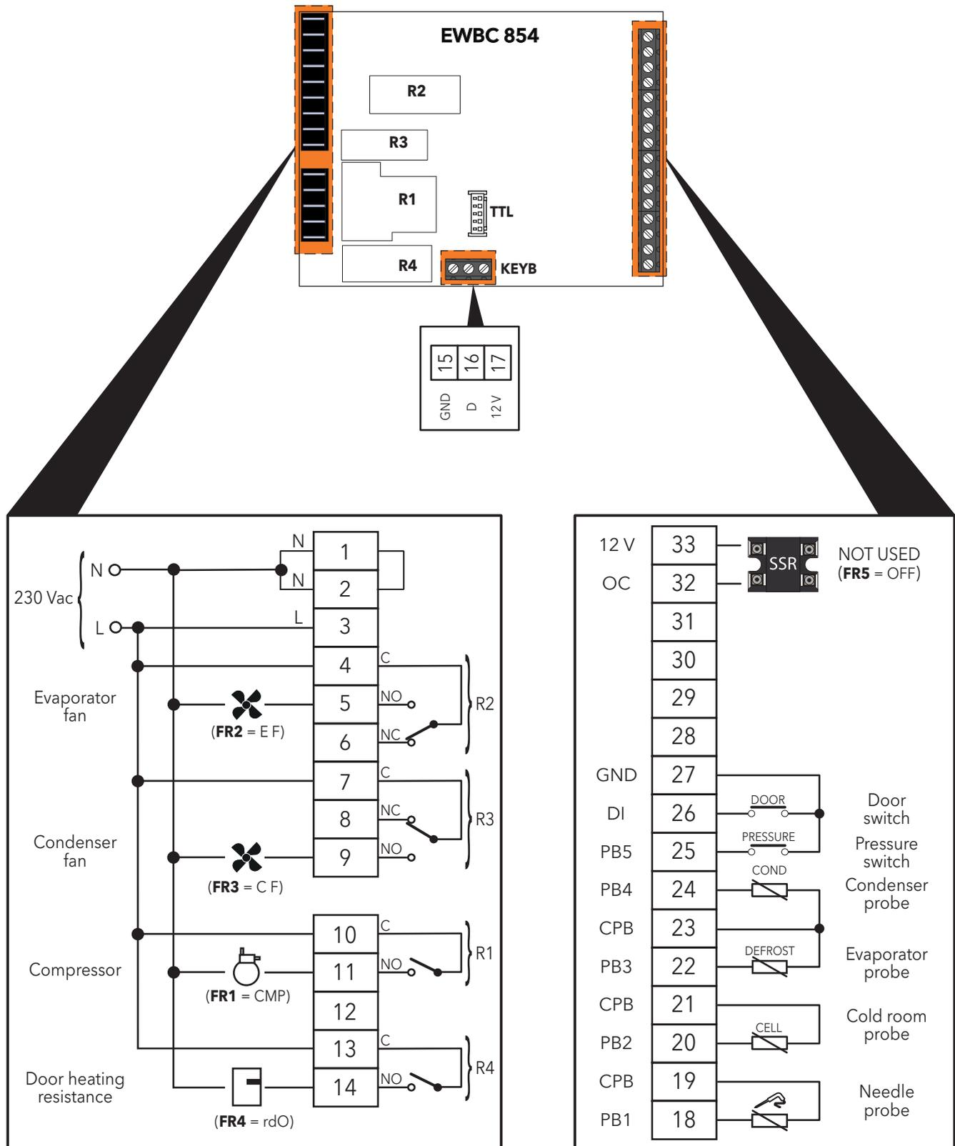
Fig. 10. EWBC 854 connection diagram example
