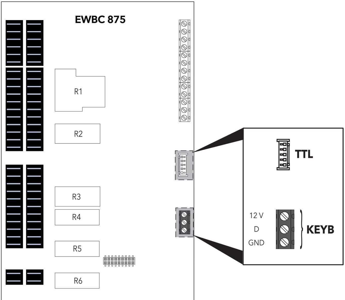
**Fig. 4.** Serial ports: TTL and KEYB
