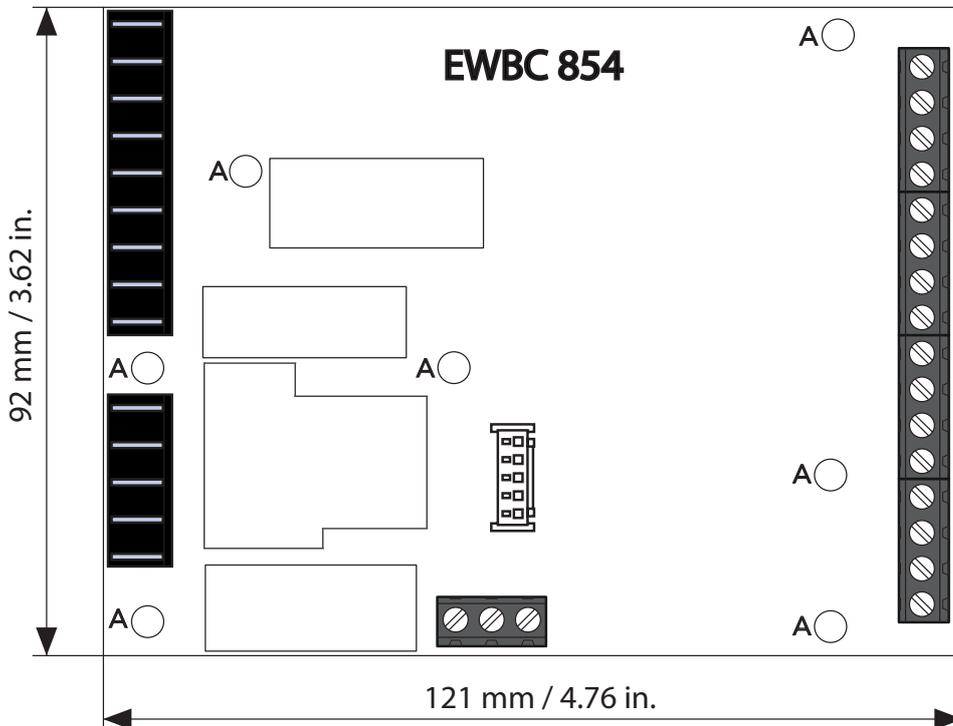
Fig. 5. EWBC 854 installation and dimensions
