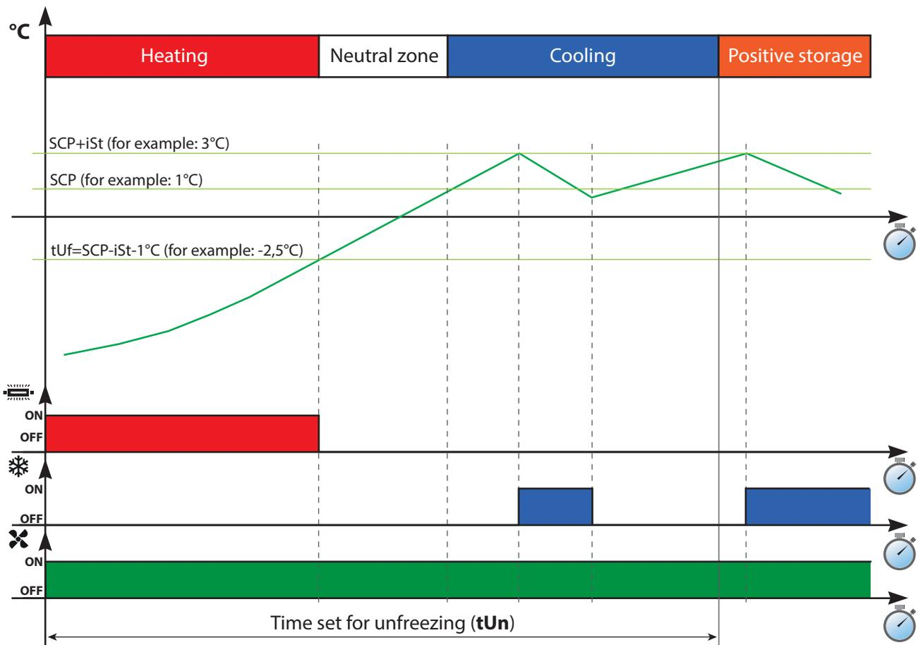
**Fig. 22.** Unfreezing cycle
