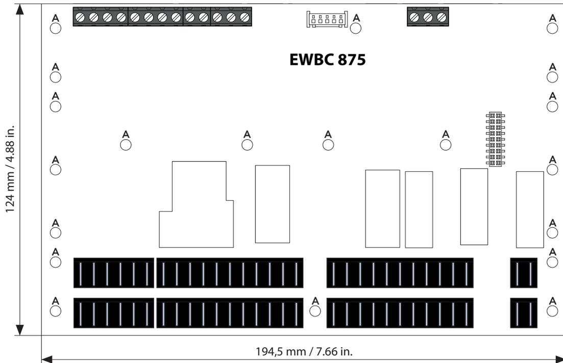
Fig. 6. EWBC 875 installation and dimensions
