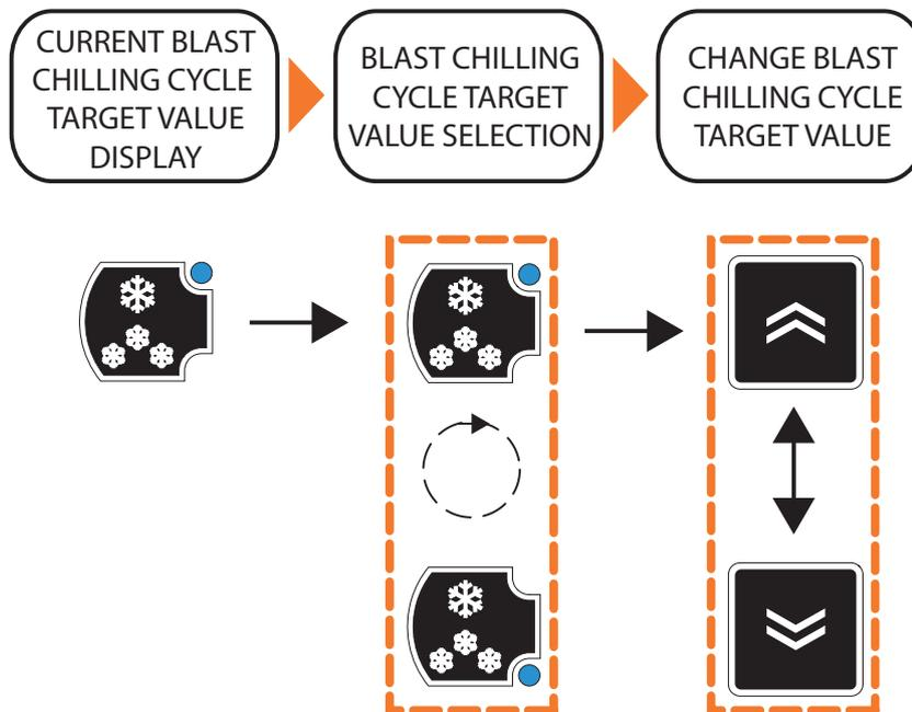
Fig. 17. Selecting a blast chilling cycle target value
