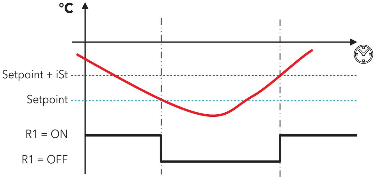
Fig. 25. Compressor operation
