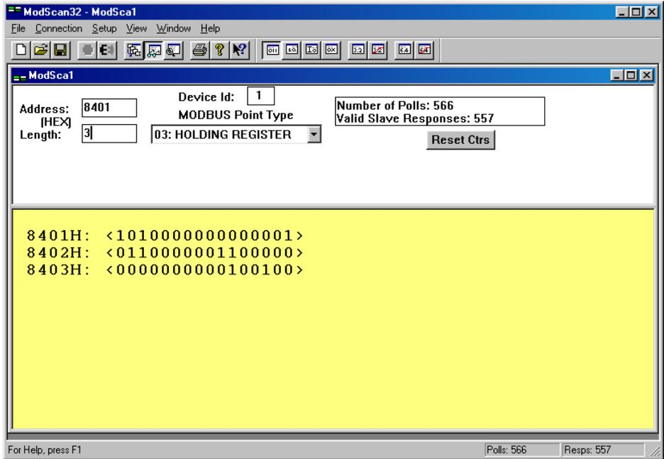
The state of all the digital inputs is read. Note that some are energized. For example IDL1, IDL14, IDL16 and IDL22 on the XTMH base + IDL1 and IDL8 on the first external expansion module + IDL1, IDL5 e IDL8 on the second external expansion module.
