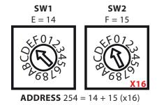
As an example, address 254 is reserved for setting the Baud rate to 9,600 bits per second.
