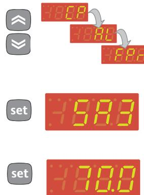
• By pressing the 'UP' and 'DOWN' keys you can scroll through all the folders in the programming menu
