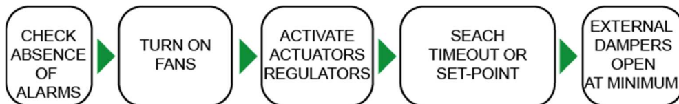
Fig 4 - Passage to ON status with making operative process
