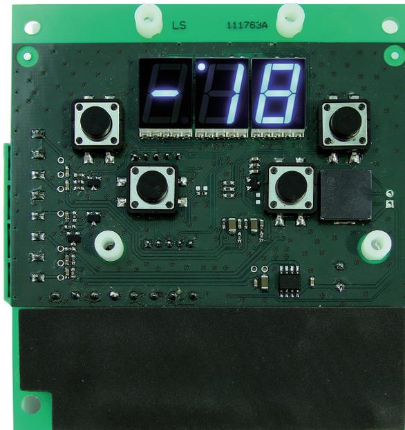
**Low End integrated controller for blast chillers**
