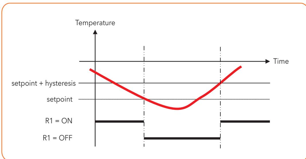
**Fig. 11.** Compressor operation
