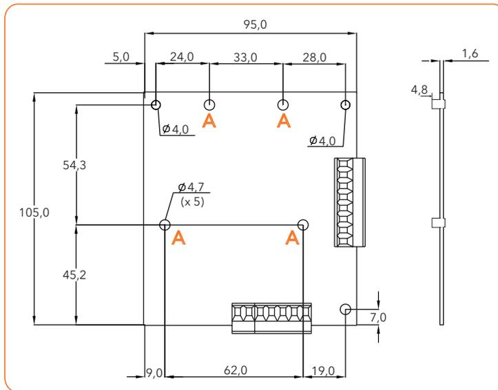
**Fig. 2.** Mechanical installation - measurements
