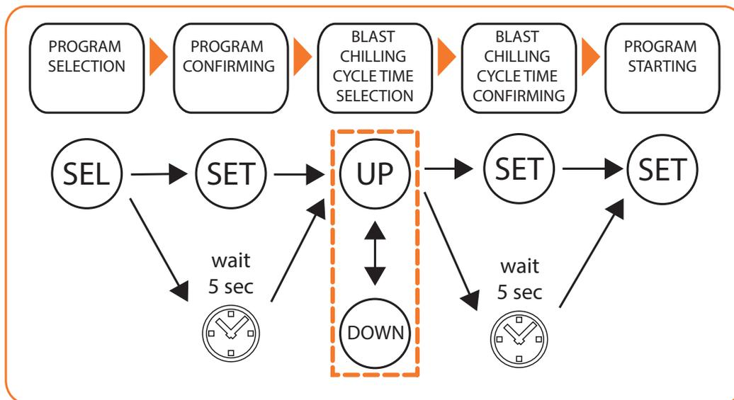
**Fig. 9.** Selecting and starting a manual program
