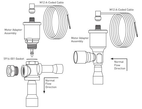
should be replaced on the valve. The cable can be installed in any of the four directions. Care should be taken to assure the pins are aligned with the connector. When tightening the cable nut, the cable nut should not be twisted or rotated.
